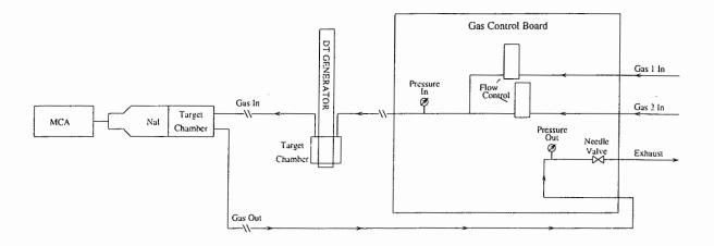
Figure 1: Experimental set-up for <sup>16</sup>N tests
