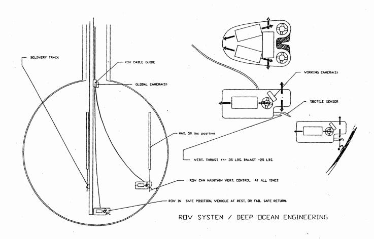
Figure 2: ROV deployment system (Deep Ocean Engineering, Inc).
