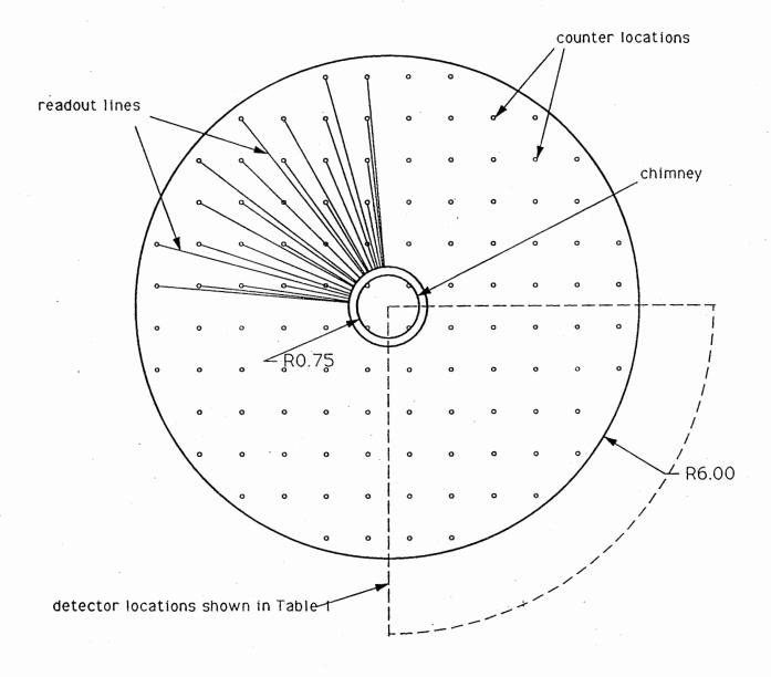
Figure 1: Plan view of the arrangement of the counter strings inside the acrylic vessel.
