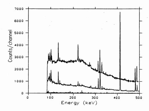
Figure 1:  $\gamma$ -ray spectrum of acrylic sample: the top curve was obtained with the germanium detector in "normal" mode; the middle curve shows the results of Compton suppression. The bottom curve shows the room background. The three curves have been normalized to the same collection time.
