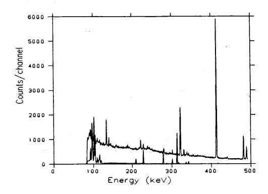
Figure 3: Compton suppressed spectrum of acrylic. (Same as middle curve in figure 1.) The lower curve is the calibration source which contained known amounts of thorium and uranium.
