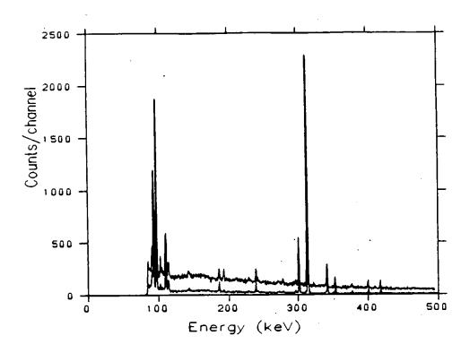
Figure 2:  $\gamma$ -Ray spectrum of chemically separated acrylic sample. Compton suppression was used to obtain the lower curve.
