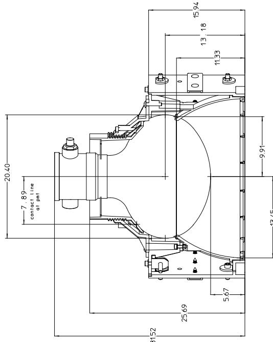
Fig. 7. Photomultiplier mounted in a hexagonal ABS cell, which also forms the light-concentrator housing. Dimensions are in cm.
