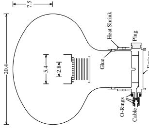
Fig. 6. A schematic of the Hamamatsu R1408 PMT and its waterproof enclosure. The 9 dynodes are shown as solid horizontal lines. The focusing grid is shown as the dashed lines above the dynodes. The volume inside the enclosure is filled with soft silicone gel. The end cap is flexible to allow for thermal expansion. The plug is sealed with heat shrink and thermal adhesive. Dimensions are in cm.
