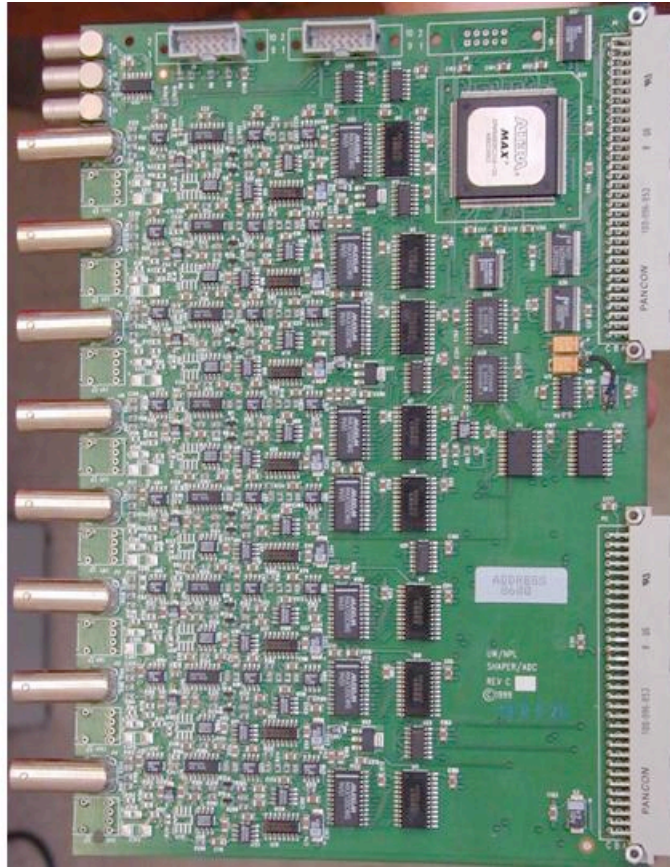
Figure 2-15: NCD Shaper/ADC board
