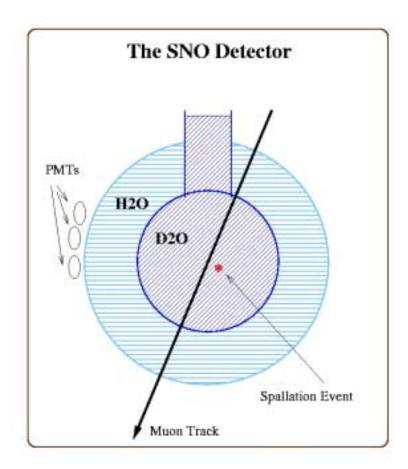
The above drawing (not to scale!) depicts muon-induced spallation in the SNO detector.
