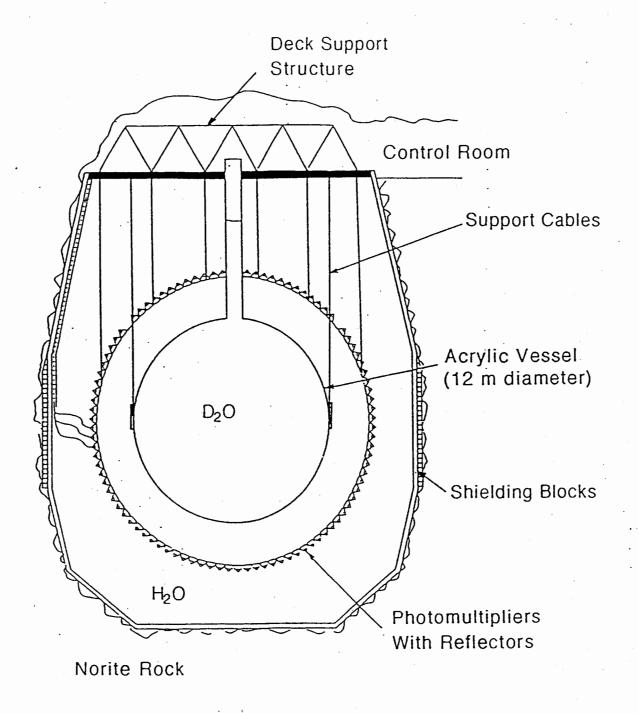
Figure 1 A cross section drawing of the SNO Neutrino Detector
