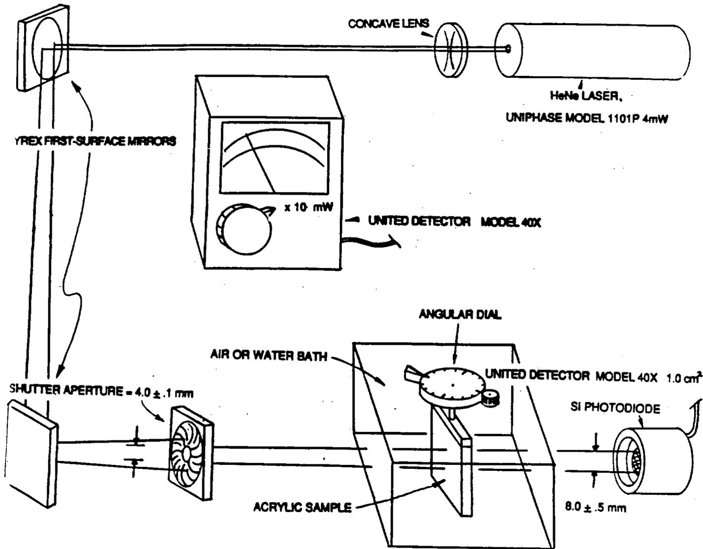
Figure 3: Schematic of experimental setup.
