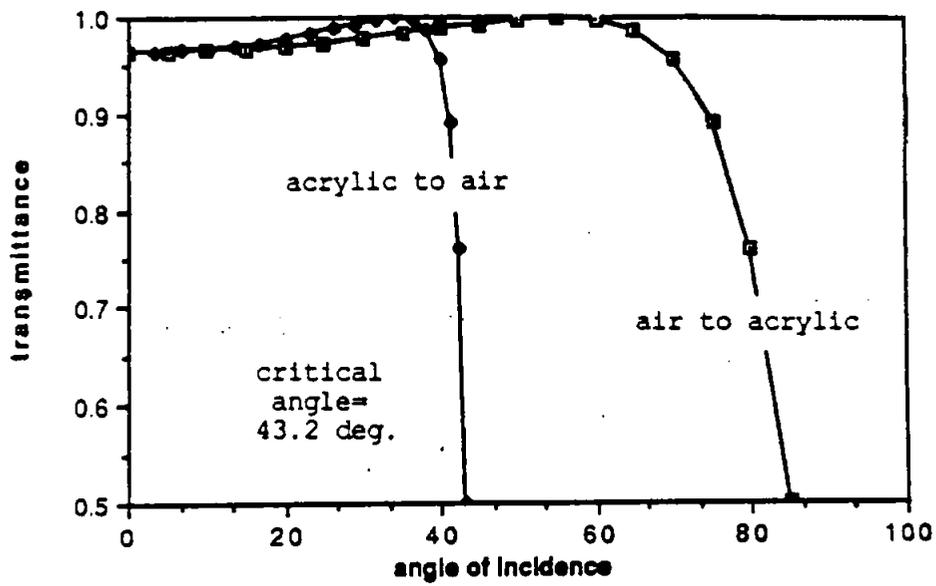
transmittance between air and acrylic, TM mode
