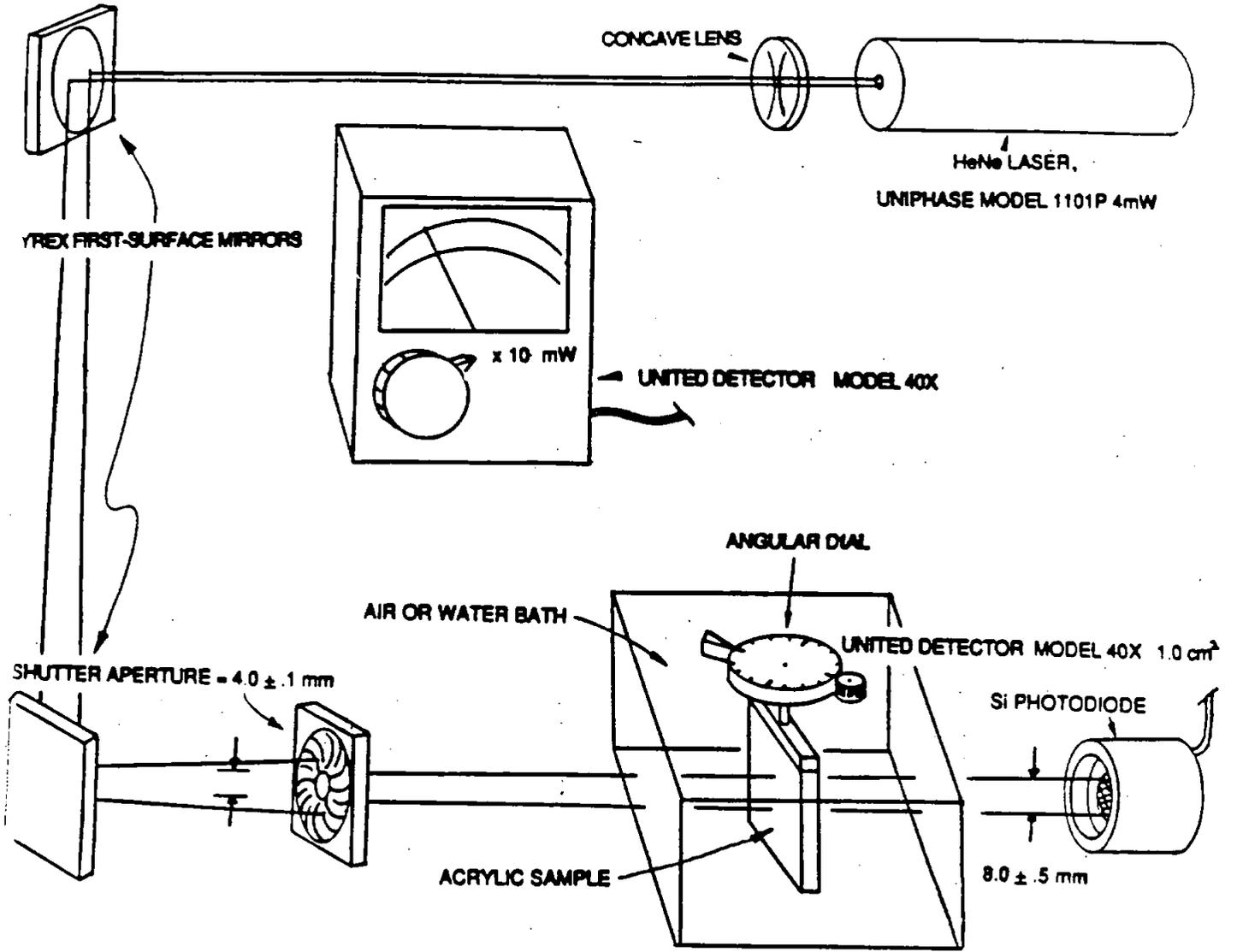
Figure 3: Schematic of experimental setup.
