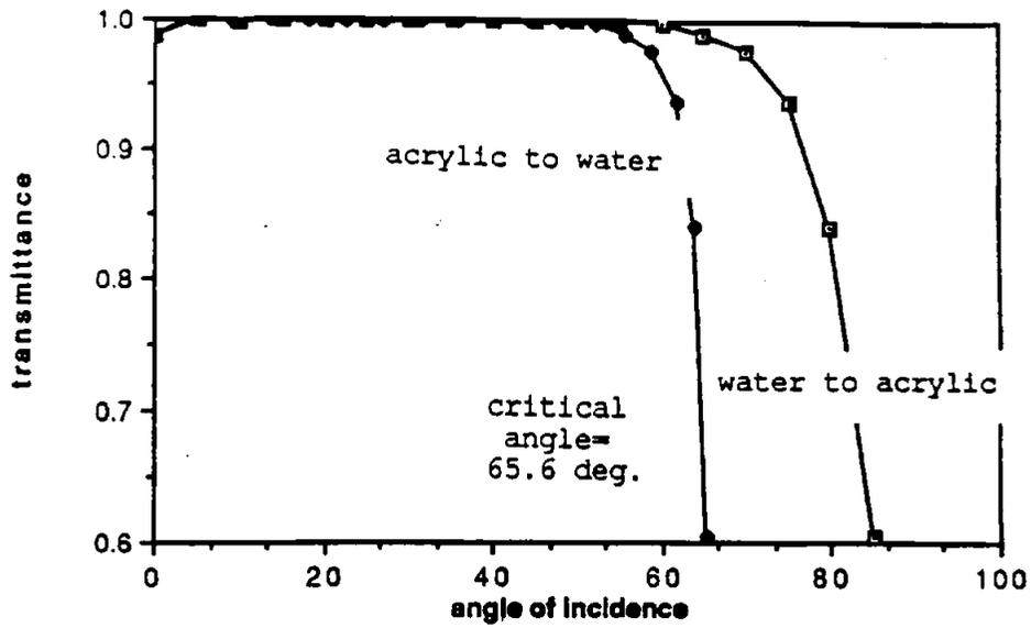
transmittance between water and acrylic as calculated using Fresnel's equations, TM mode
