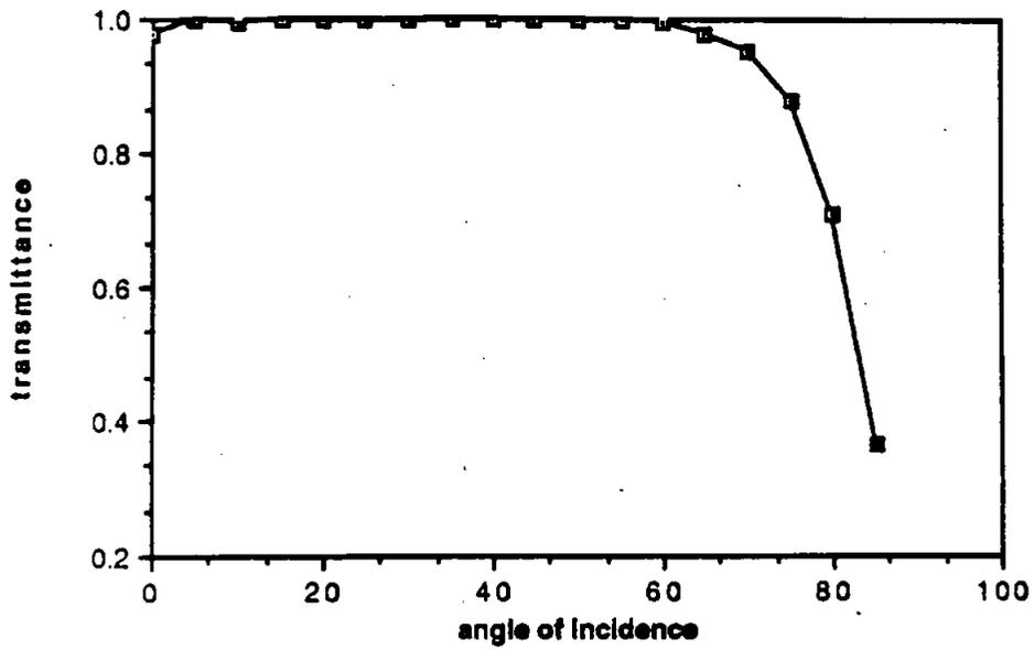
transmittance in uncrazed acrylic in water
