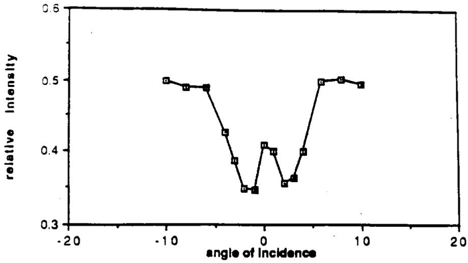
A4, small angle, demonstrates spike at 0 degrees not apparent on other graph
