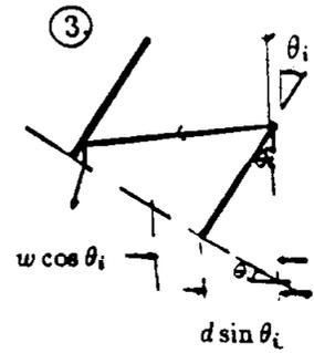
$$\textcircled{1} T = \left( \frac{w \cos \theta_i - d \sin \theta_i}{w \cos \theta_i} \right) (T_{b \rightarrow ac})(T_{ac \rightarrow b}) = \left( 1 - \frac{d}{w} \tan \theta_i \right) (T_{b \rightarrow ac})^2$$
