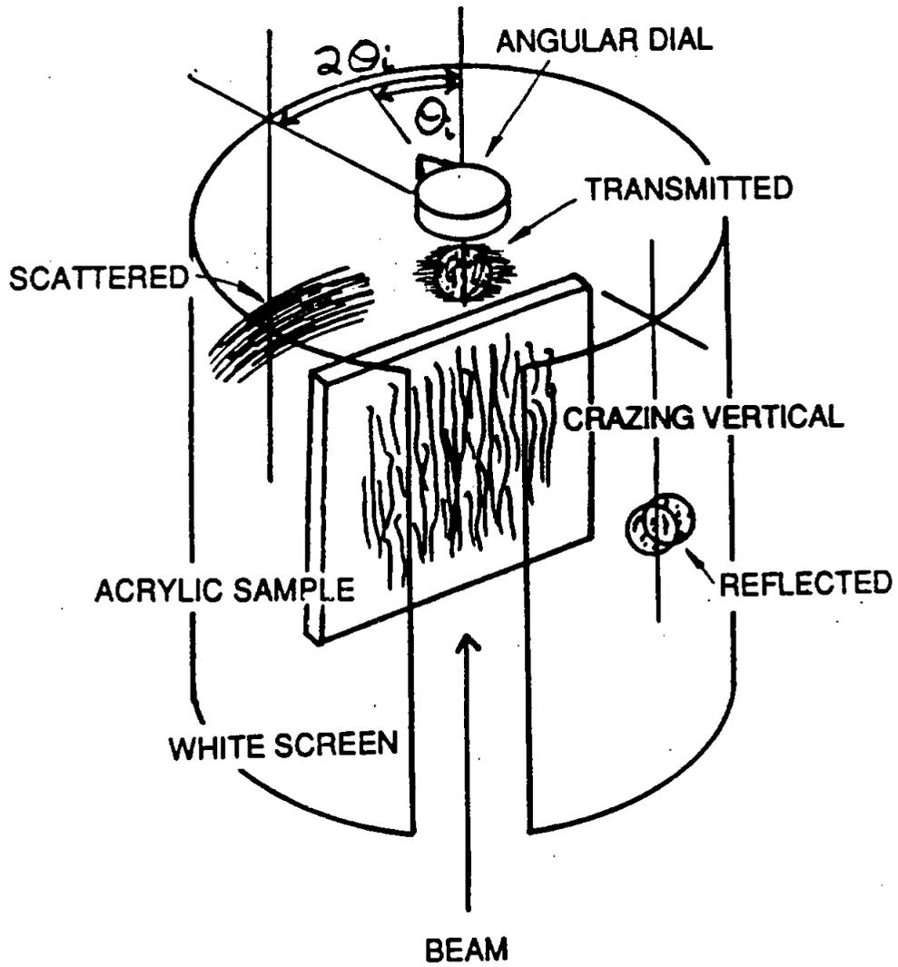
Figure 4: Effect of crazing on incident light beam.
