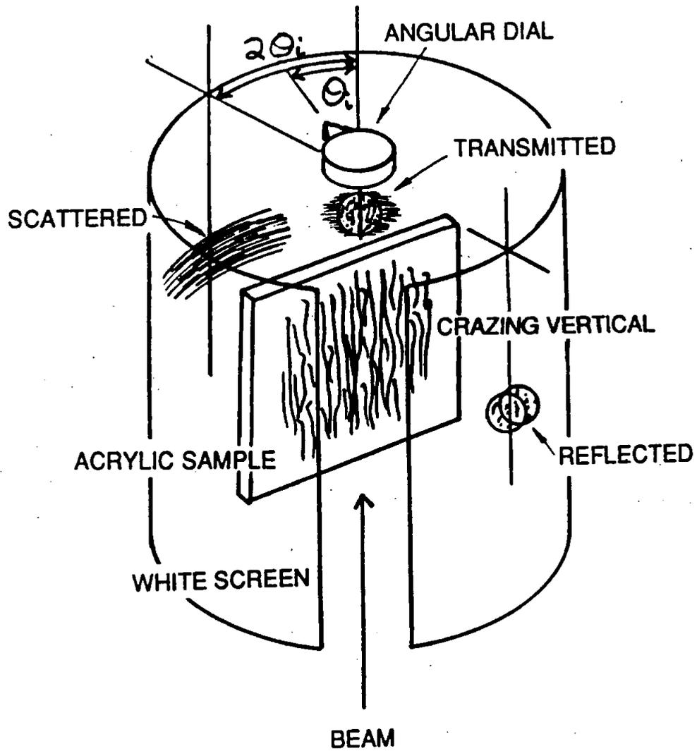
Figure 4: Effect of crazing on incident light beam.
