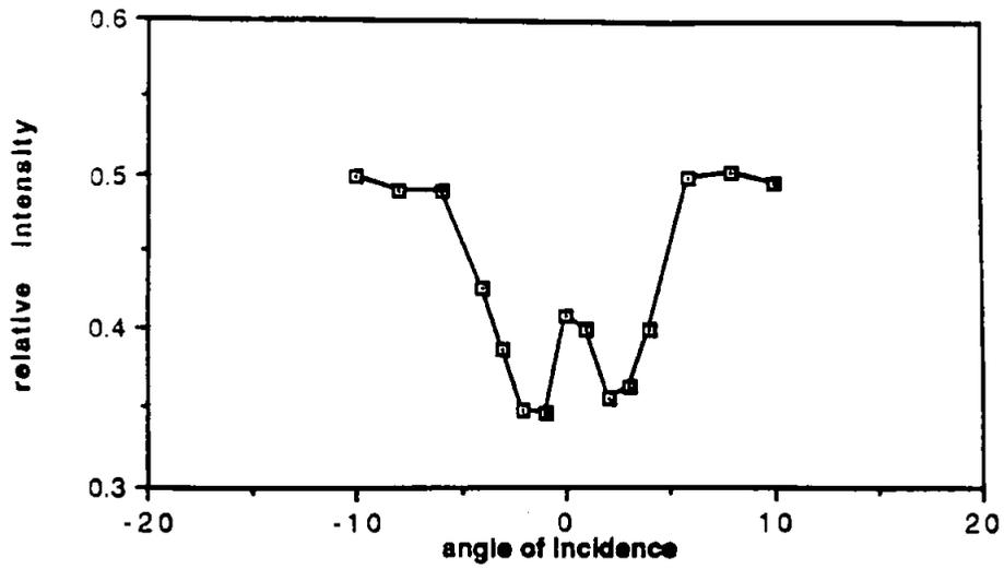
A4, small angle, demonstrates spike at 0 degrees not apparent on other graph
