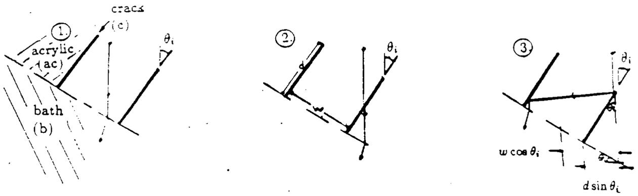
$$\textcircled{1} T = \left( \frac{w \cos \theta_i - d \sin \theta_i}{w \cos \theta_i} \right) (T_{b \rightarrow ac})(T_{ac \rightarrow b}) = \left( 1 - \frac{d}{w} \tan \theta_i \right) (T_{b \rightarrow ac})^2$$
