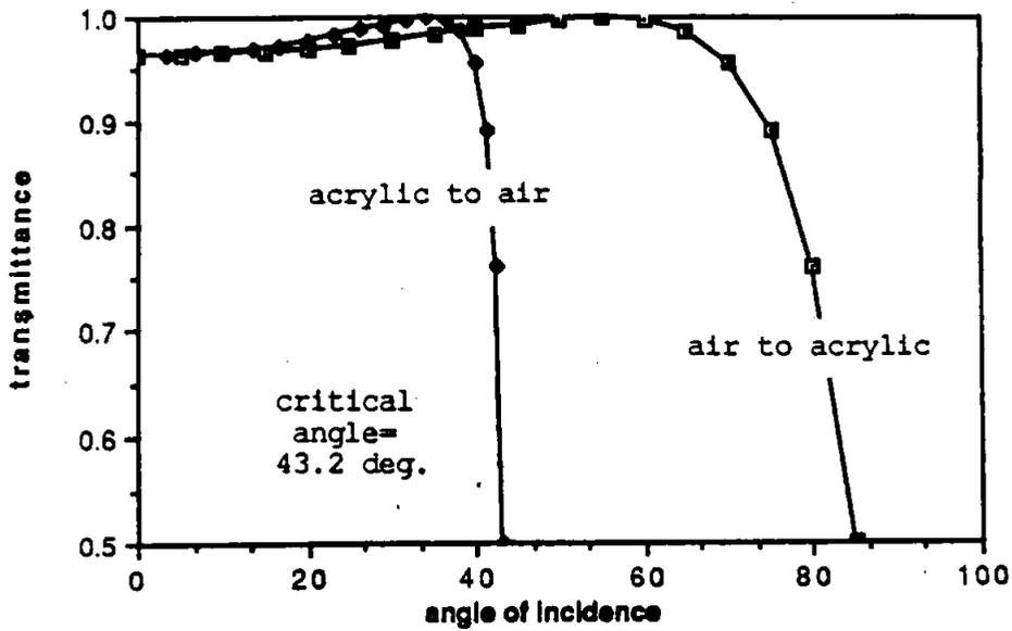
transmittance between air and acrylic, TM mode
