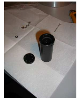
Figure 3.4: Delrin canister deployed into the center of the AV. Left: drawing of the inner and outer cans; right: photo with the inner can inside of the outer can.
