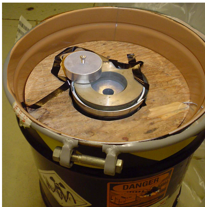
Figure 4.1: Barrel used to transport the ^{24}\text{Na} source from Queen's to Sudbury. Contained a heavymet castle which had 2 inch thick walls.
