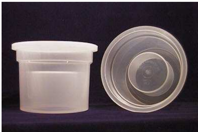
Figure 3.5: Marinelli beaker used to measure ^{24}\text{Na} source with the underground germanium detector.
