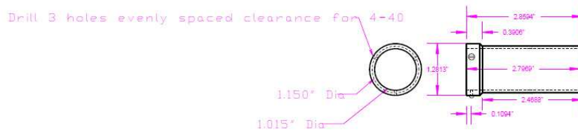
Figure 3.4: Delrin canister deployed into the center of the AV. Left: drawing of the inner and outer cans; right: photo with the inner can inside of the outer can.
