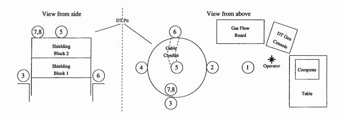
Figure 2: Radiation Survey Measurement Points.
