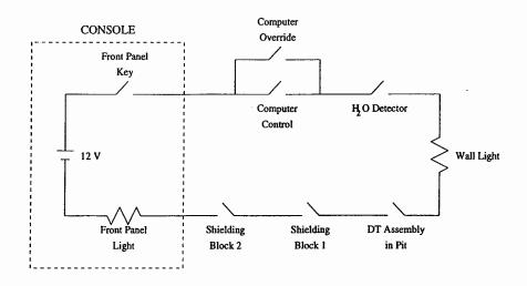
Figure 1: Schematic of Interlock System.
