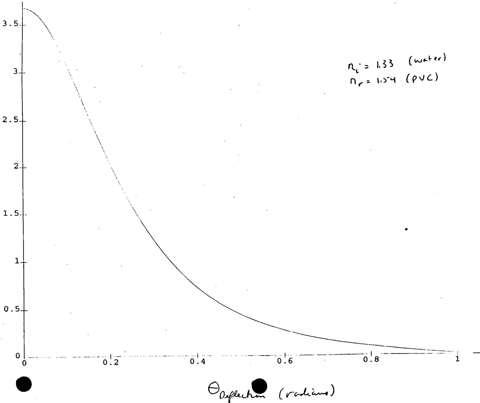
Transmission polarization perpendicular
