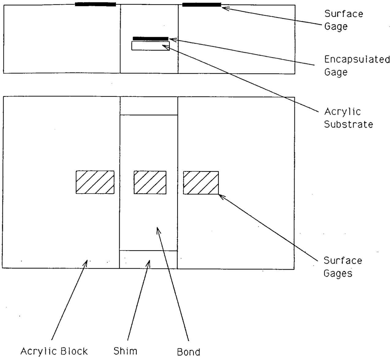
Figure 1: Schematic of a bond joint showing location of stress gages.
